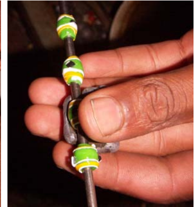
Step 3 With the use of a small metal mould, the bead is getting its final shape.
