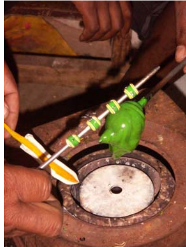
Step 2 Selected colours are combined while the plastic is being heated. The bead is gradually built-up.
